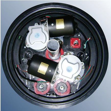
Front view of IGDU unit showing twin 24 Volts DC motors, limit setting cams etc.
